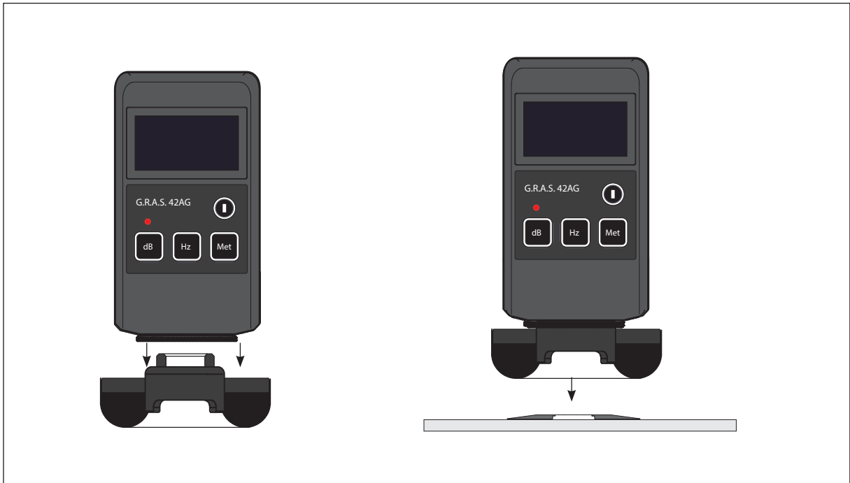
Fig. 8. In-situ verification using 42AG and RA4800.
